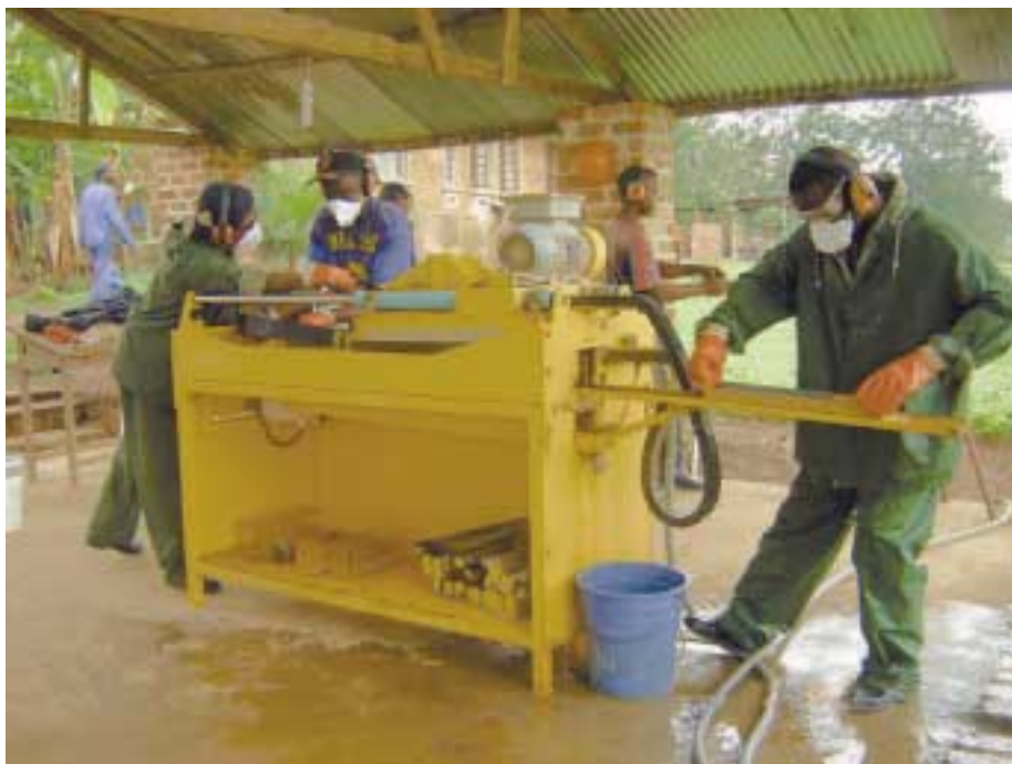
Cutting core at Namoya with an Almonte core saw
