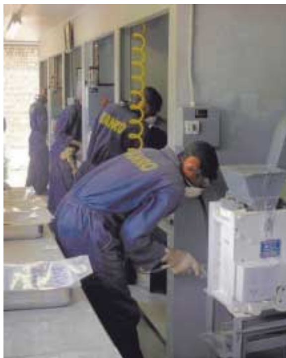
Crushing and pulverising samples in the Bukavu facility
