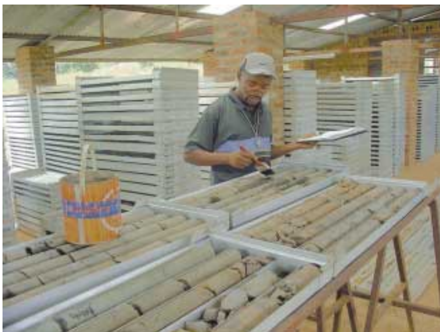
Checking and logging core at Namoya
